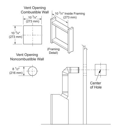
Figure 9 - Vent Opening Requirements
